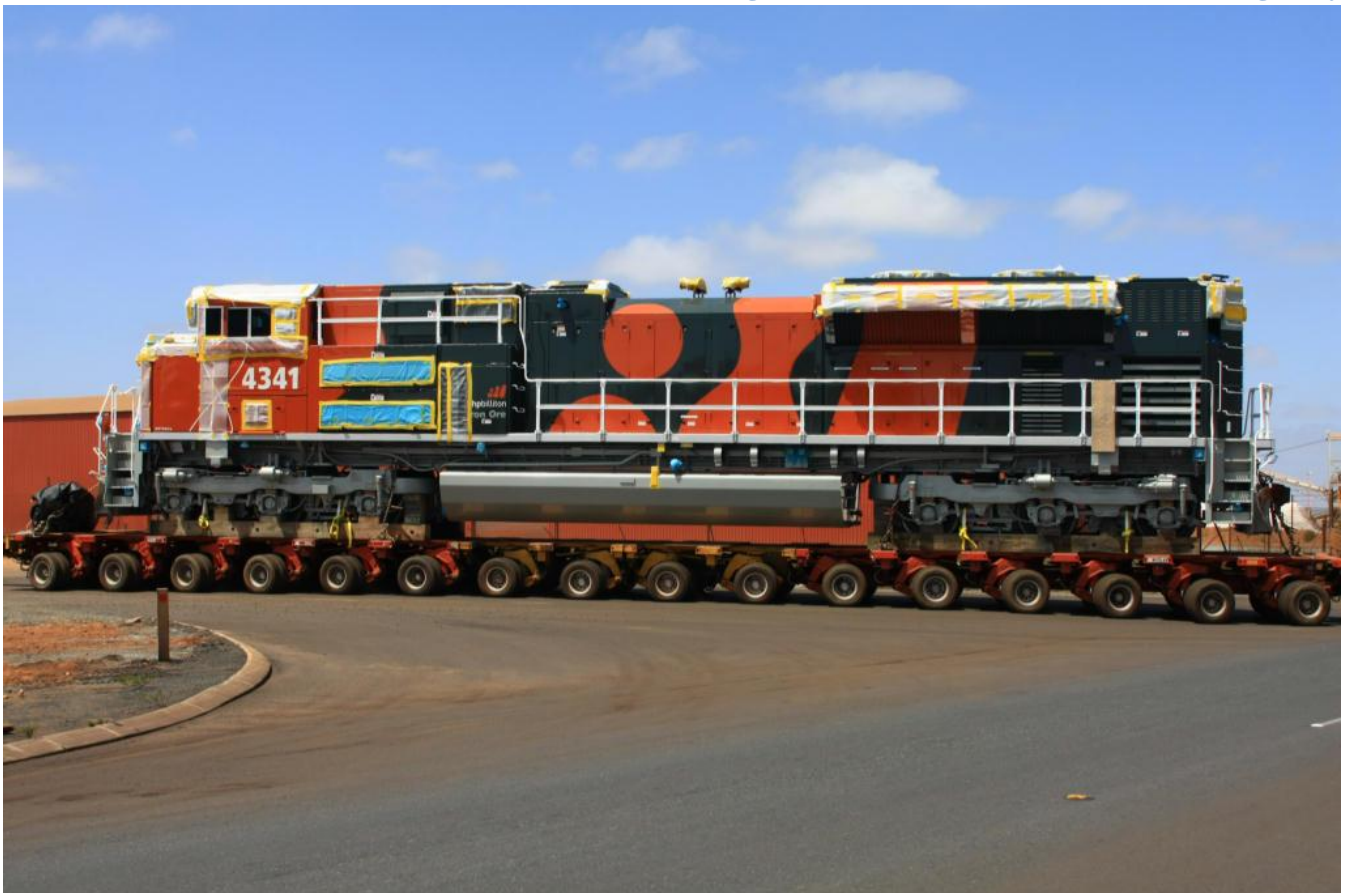
Side on shot of 4341 as it turns off Gilbert Street and enters the Nelson Point complex through gate #9 note wooden brackets under bogies allowing locomotives to be shipped complete. Photo Toad Montgomery
