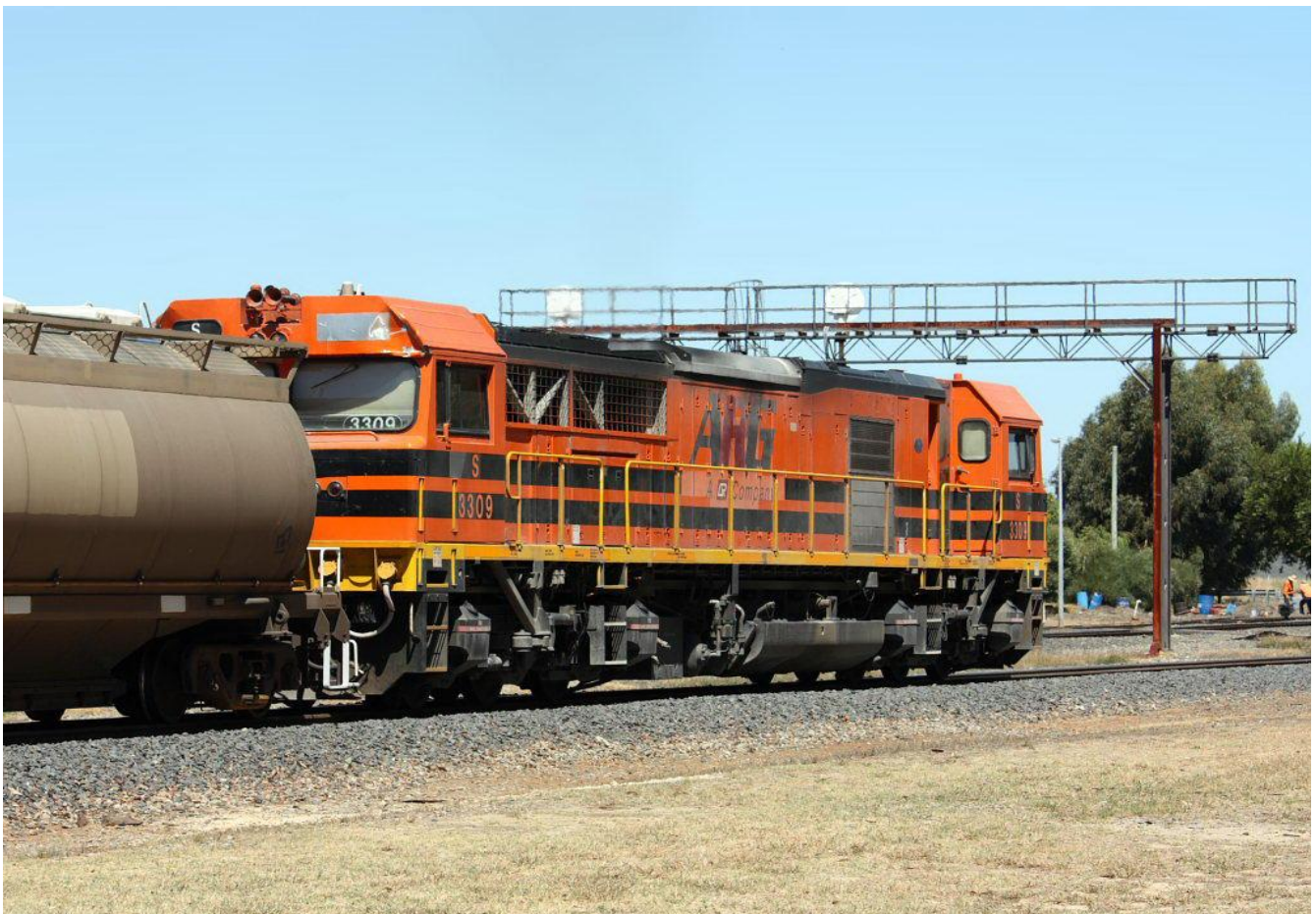
S3309 at Brunswick March 6th appears to have suffered cab damage on both top left and top right above the cab windows this may have been caused by a loading chute coming down early. Photo Stuart Jackson
