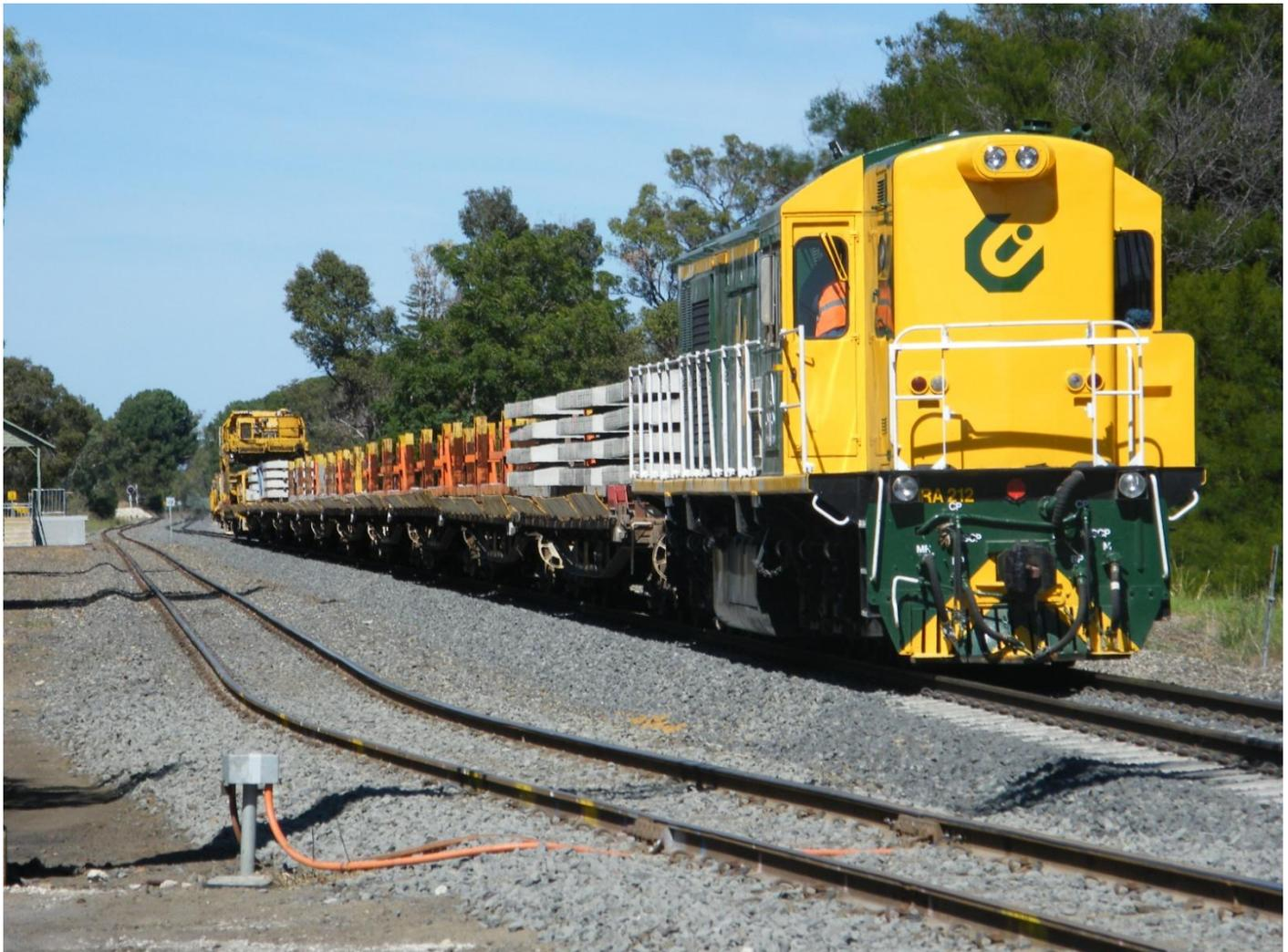
RA212 and tracklaying train sitting on main line at Waroona following completion of laying final section of concrete sleepers between Kwinana and Bunbury on South West Main line on April 6th. Photo Jim Bisdee
