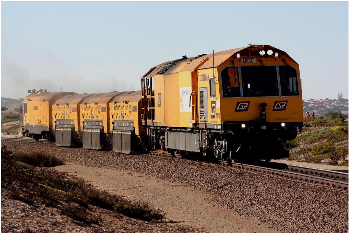
QR rail grinder MMY32 grinding the track on the Narngulu yard-Geraldton port line at the west end of the City of Geraldton on April 26th. Photo Phil Melling
