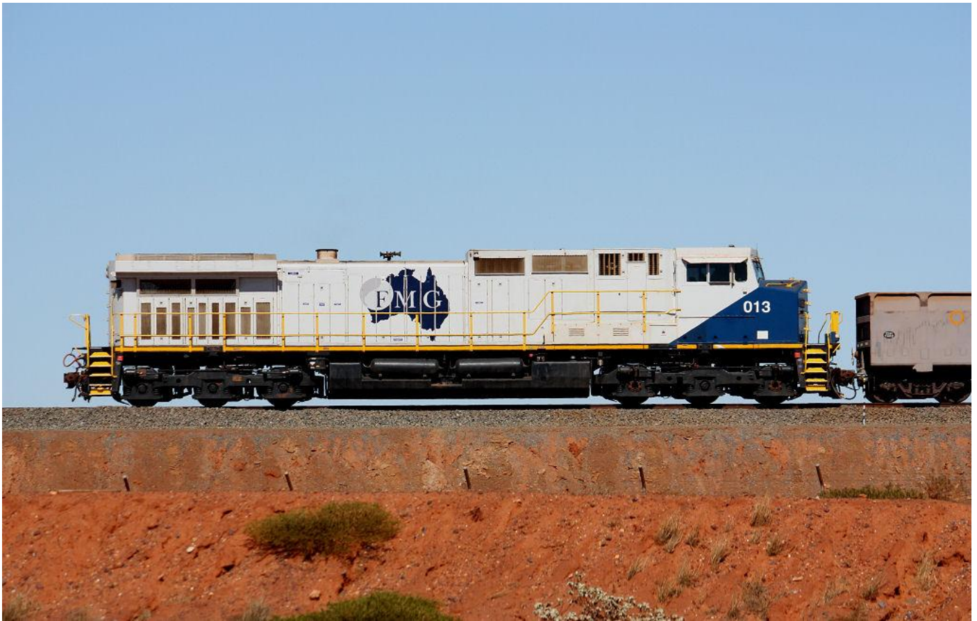
Fortescue Mining Group General Electric CW44-9 locomotive 013 is yard shunter at FMG unloader and port at southern end of Port Hedland harbour on July 16th.
