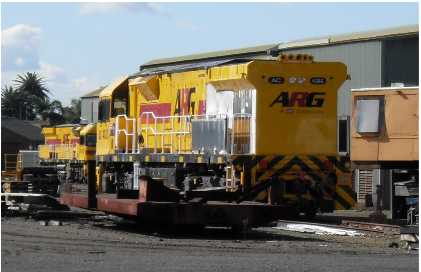
AC4302 showing where steel panels have been removed from long hood under radiators and are being substituted with aluminium panels in effort to reduce the locomotives weight July 30th. Photo Brad Coulter
