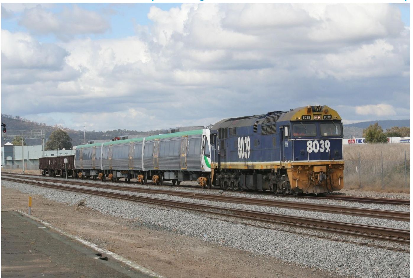
8039 hauls EMU set #85 and three gondola wagons for braking that also contain the narrow gauge power bogies through Midland loop on 5th on way to old workshops for gauge conversion. Photo Justin Brown
