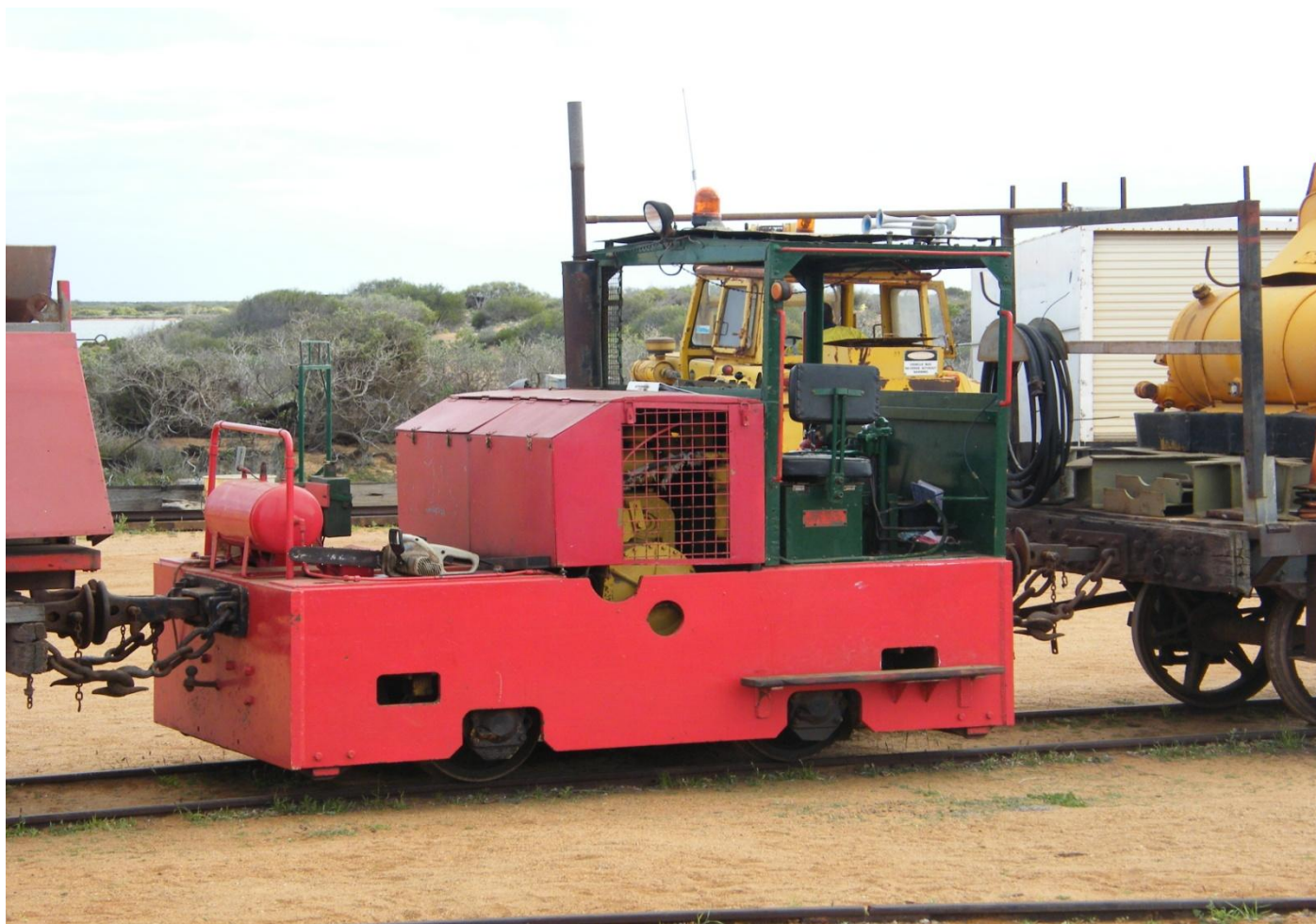
PW28 in the yards at Carnarvon Jetty on August 18th showing the changes made to the original Motor Rail Ltd Simplex locomotive now with Perkins diesel engine and automatic transmission. Photo Jim Bisdee
