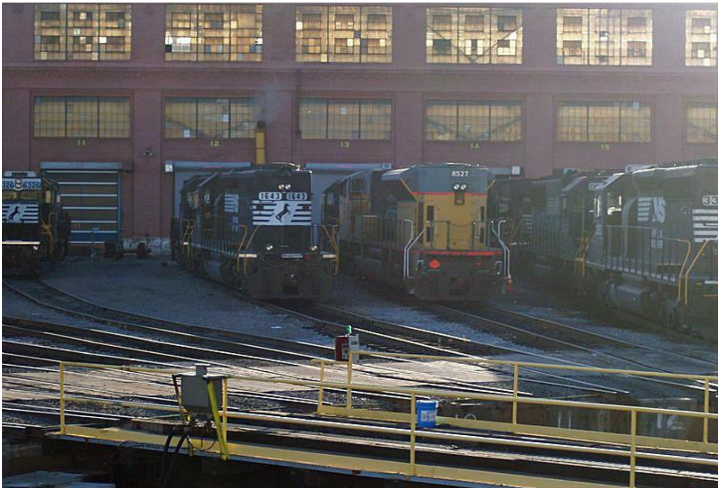
GTLX8527 former Union Pacific SD90AC-H now owned by FMG being converted to SD70AC type by Norfolk Southern at Juniata shops here with NS units near back shops November 14th. Photo Megan Salter
