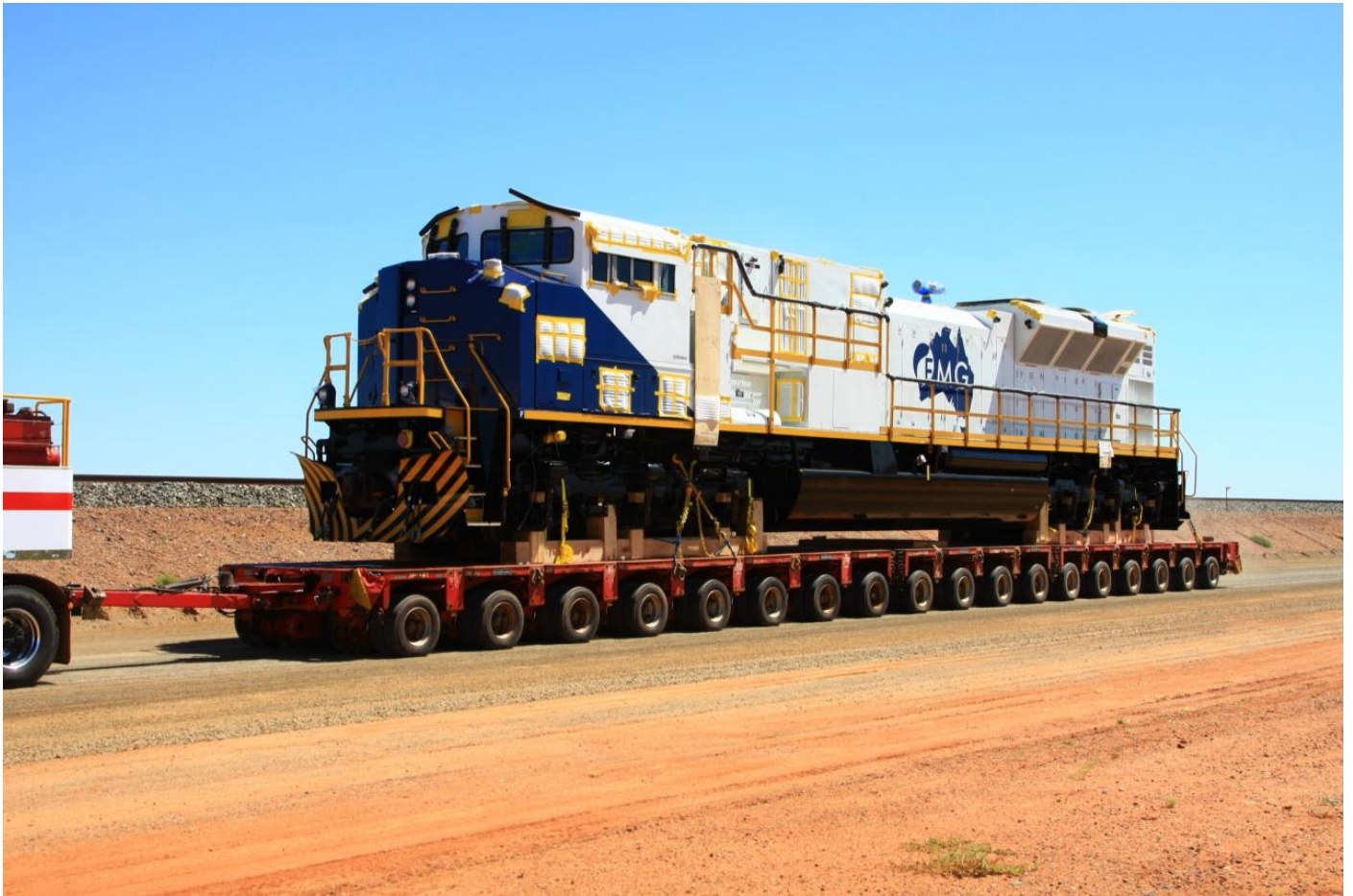
FMG901 first of four SD90MAC-H locomotives to arrive on a 144 wheel low loader at 8km on April 17th.
