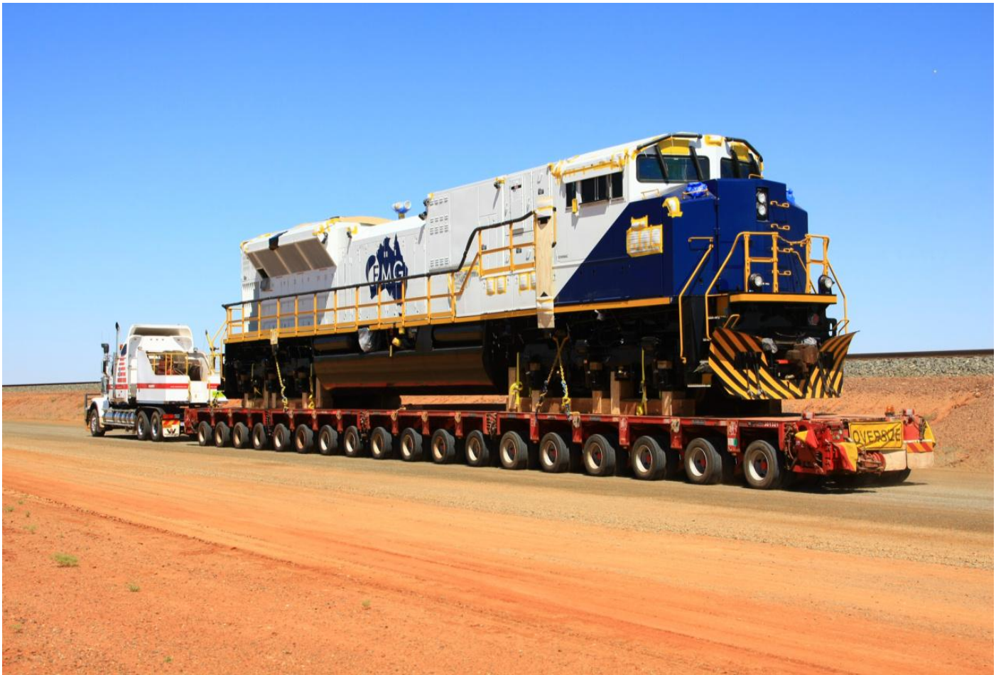
FMG SD90MAC-H 903 on 144 wheel float on April 17th.
