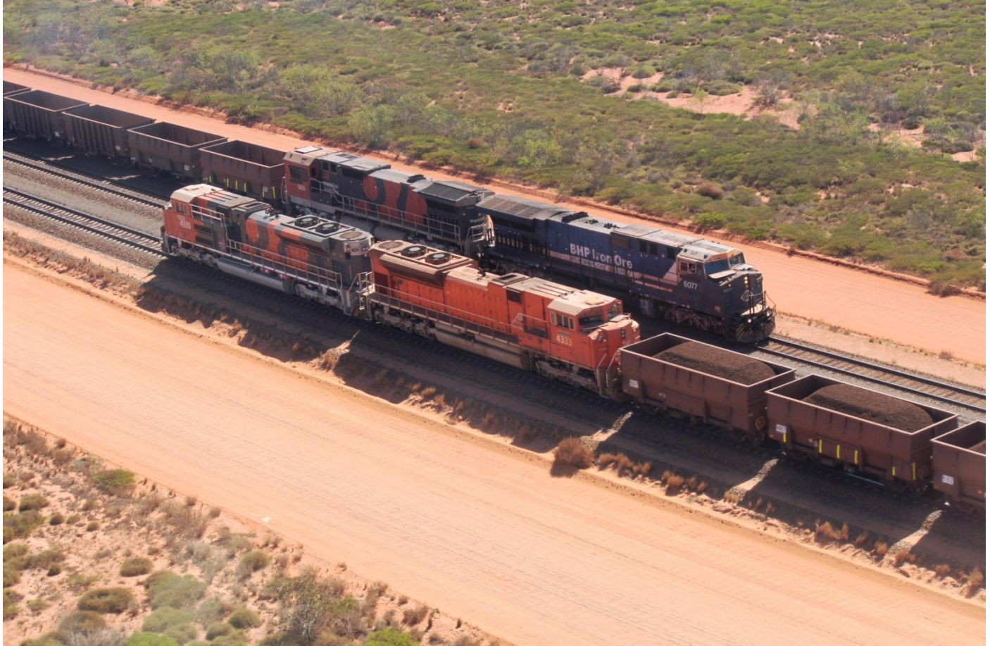
4335 & 4333 SD70ACes on loaded ore train crossing 6077 AC6000W & 5655 CM40-8M on empty at Bing that has all BHPBIO locomotive types in service in this aerial shot October 15th. Photo Baden Tidd
