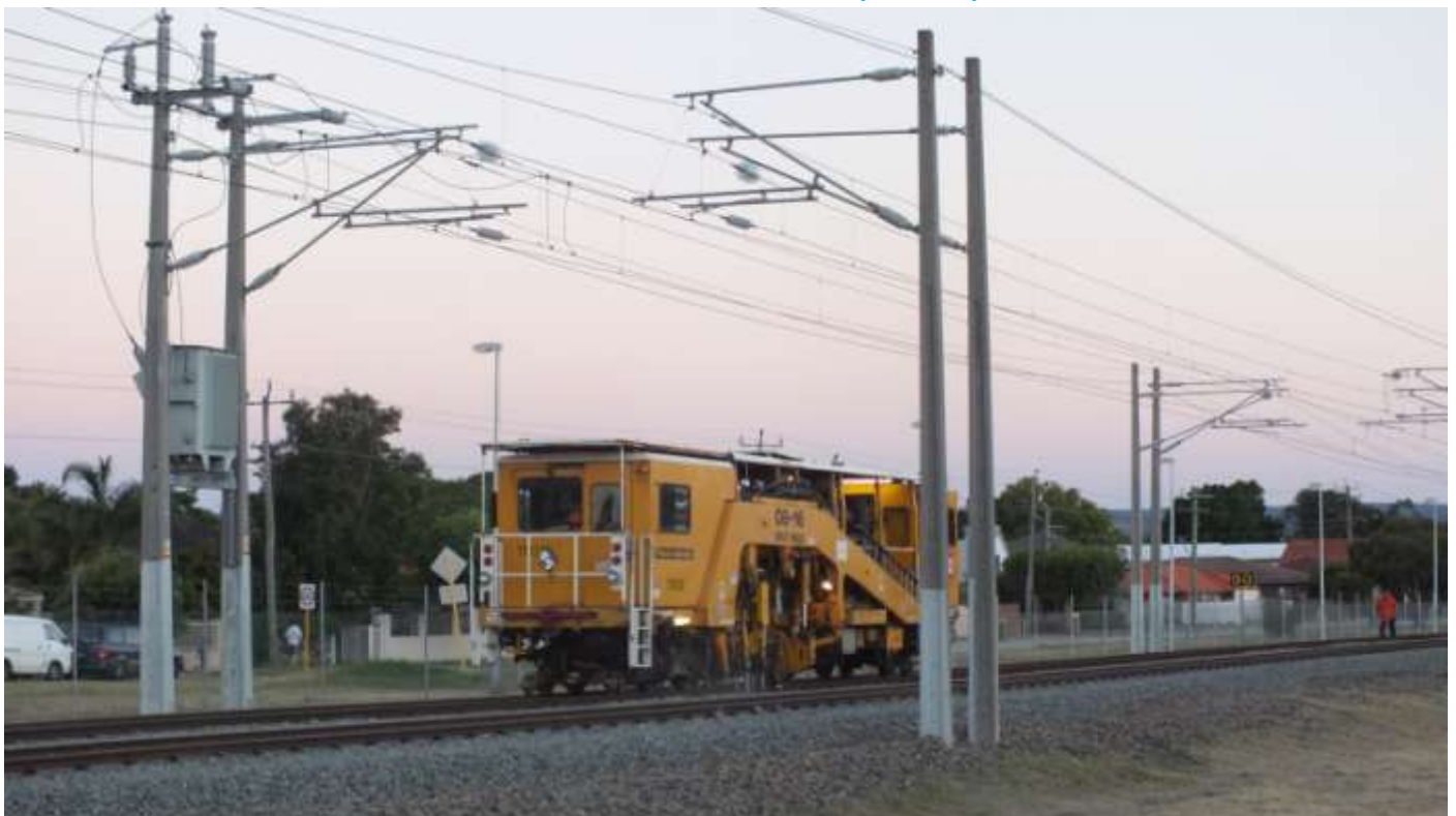
TM729 split head tamper works on the Armadale line north of Queens Park January 14th. Photo Jim Bisdee
