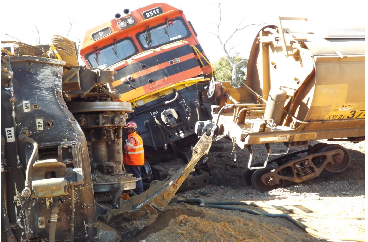
Pumping fuel out of P2505 May 18th as its fuel tank was ruptured in derailment on 17th. Photo Bill Ashman
