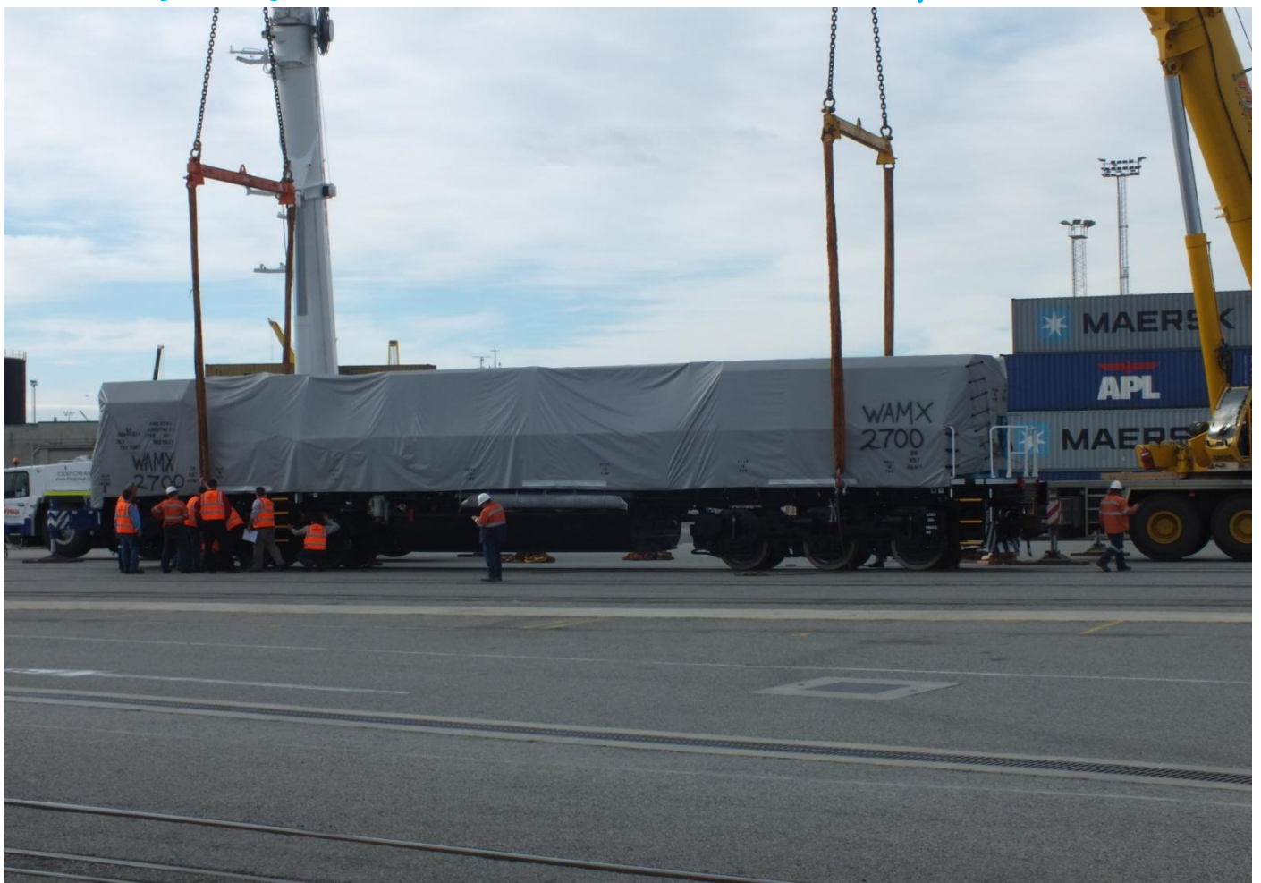
WAMX2700 [CBH001] being lowered on to its bogies May 17th at North Port. Photo Jim Bisdee
