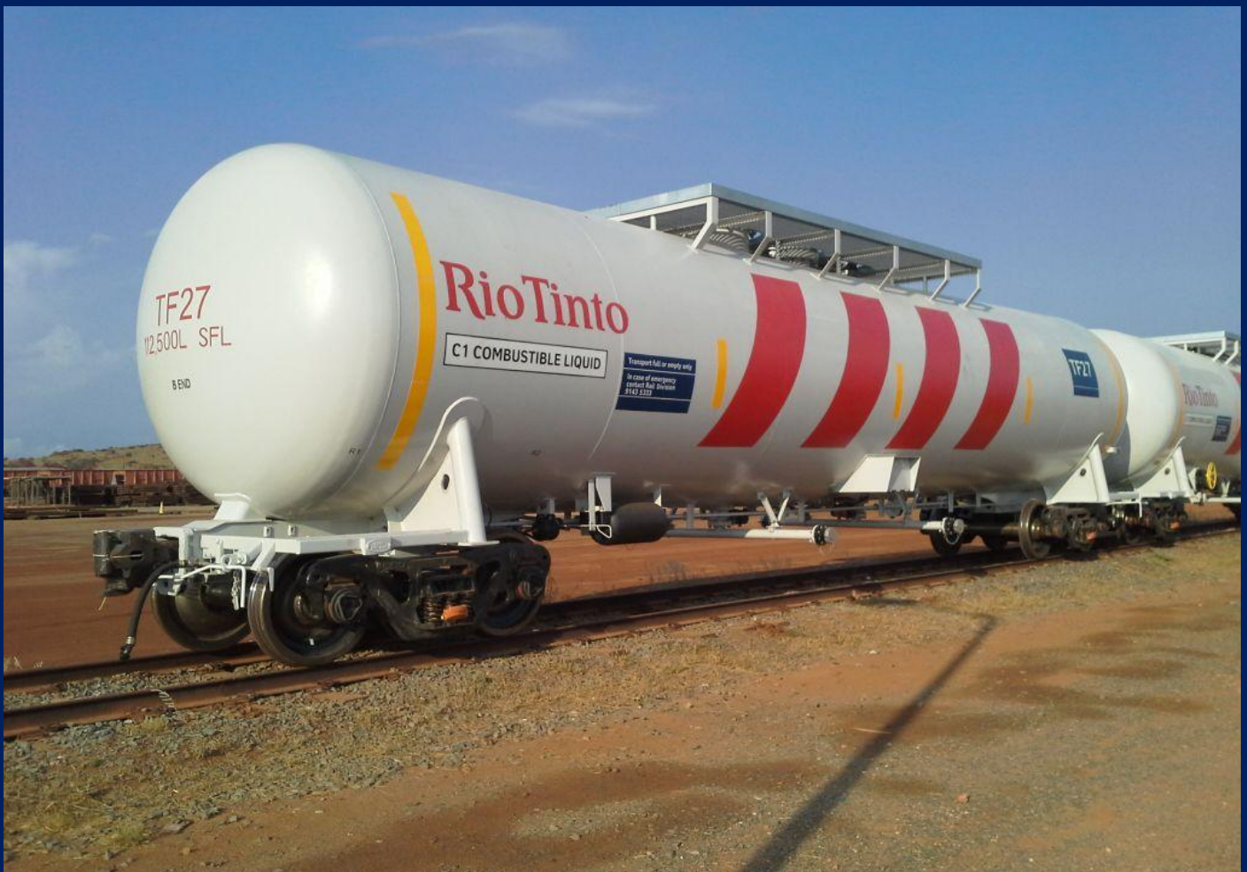
TF27 one of 32 new 112,500litre Rio Tinto tankers built by CRS China, Dampier 26/10/13. Photo Garry Lamb
