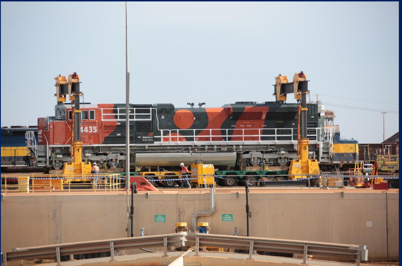
New SD70ACe being lifted off transport float at Nelson Point on 25/1.
