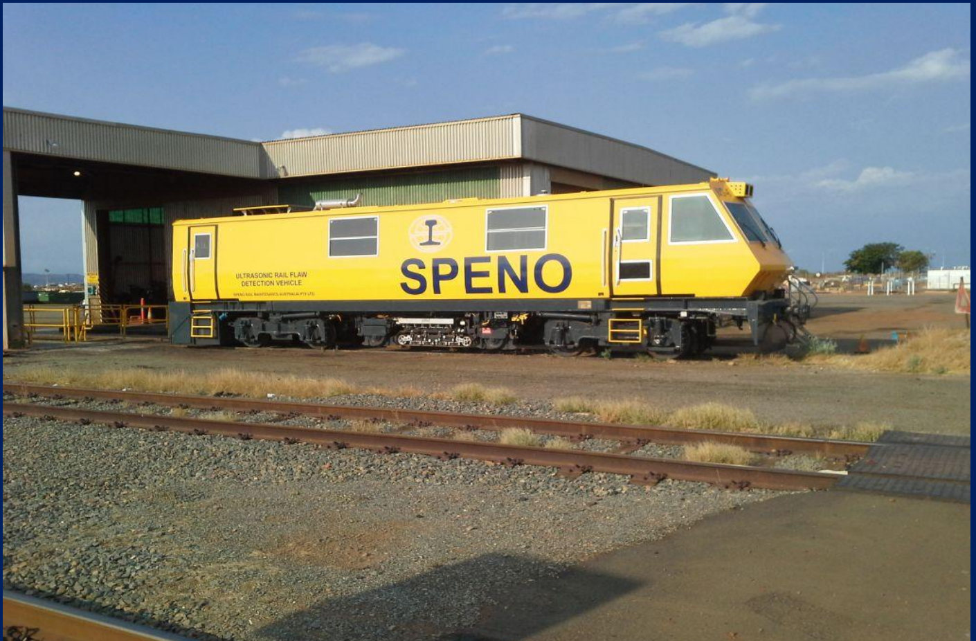
Speno ultrasonic rail flaw detection vehicle at Speno workshop 7 Mile Dampier on October 26th 2013.
