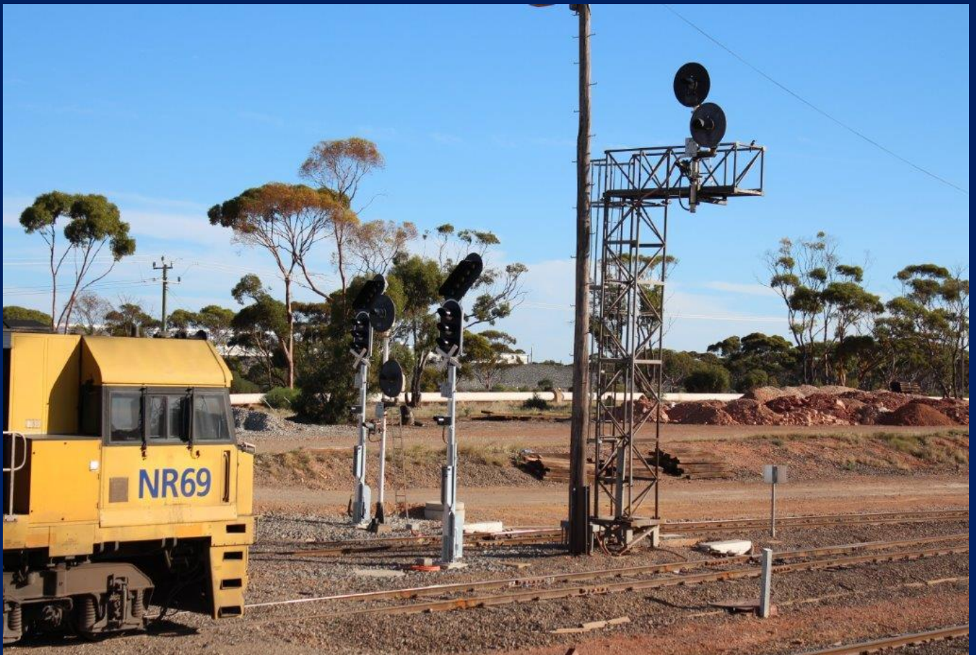
New three light signalling replacing searchlight signals at west end WEK yard 12/3.
