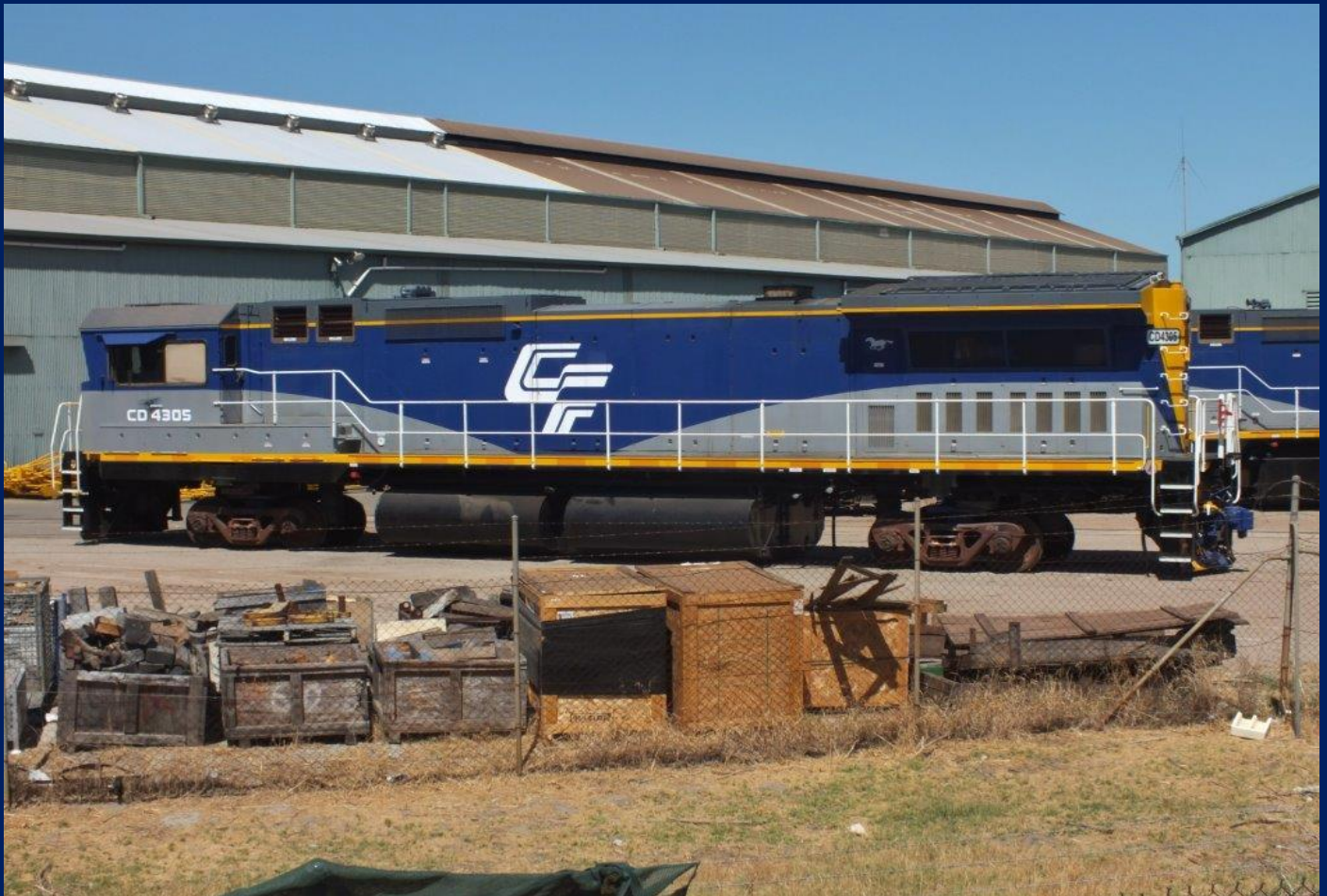
CFCLA CM40-8M CD4305 on works bogies in UGL yard Bassendean March 16th.
