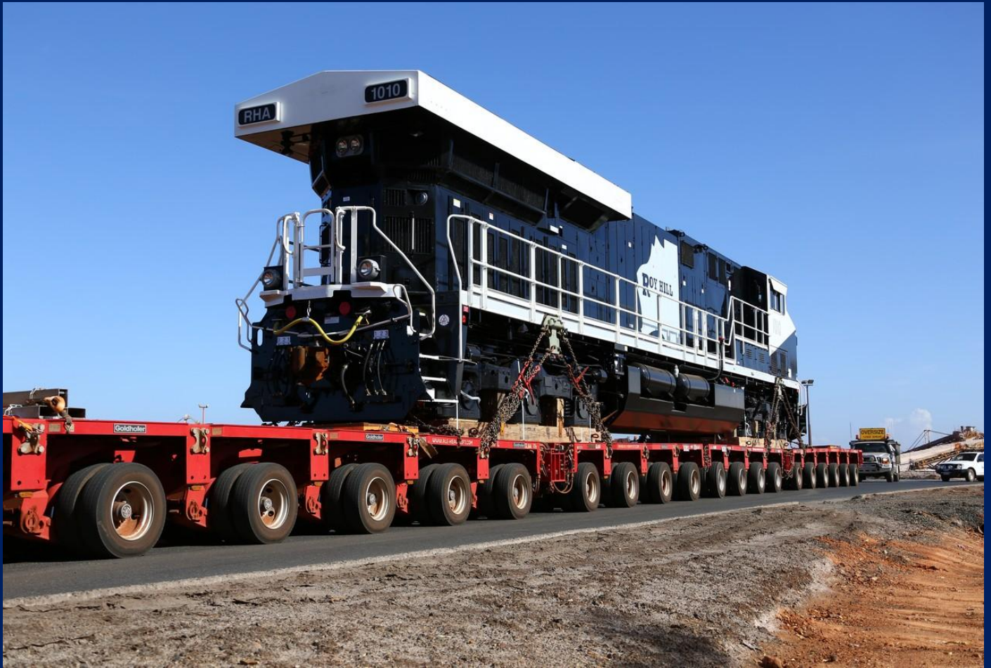
B end of ES44ACi RHA1010 with huge radiators to cope with heat in Pilbara 30/1. Photo Toad Montgomery
